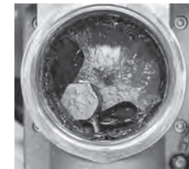
Fig. 15 - If ridge of lubricant measures 1/8" or less, add a small amount. At maximum level it should measure 1/4".
